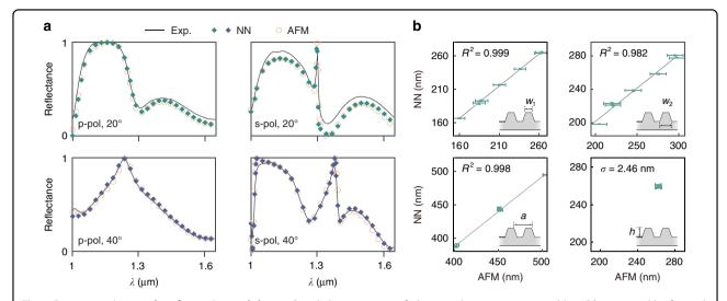
**Fig. 4 Reconstruction results of experimental data. a** Detailed comparisons of photonic dispersions: measured by ARS, generated by forward-mapping NN using optimal parameters, and simulated by RCWA using AFM measured parameters. Spectra at two incident angles (20° and 40°) with p/s-polarizations are plotted. **b** Correlations between the results of forward-mapping algorithm (green marks) and AFM measurements (gray line). Error bars are 1 σ
