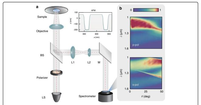
Fig. 3 Experimental setup and measured results of an SOI grating. a Schematic layout of the home-made ARS. Sample profile of the grating in the top inset. BS beam splitter, L1, L2 lenses, M mirror, LS light source. b Dispersions of the sample measured as angle-resolved reflectance (R) spectra
